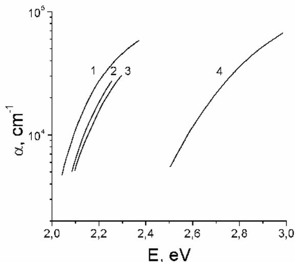
**Fig. 2.** Optical absorption spectra: 1– for homogeneous, 500 nm thick Se layer; 2– for 900 nm thick Se/As<sub>2</sub>S<sub>3</sub> NML as deposited; 3– Se/As<sub>2</sub>S<sub>3</sub> NML irradiated; 4– homogeneous 500 nm thick As<sub>2</sub>S<sub>3</sub> layer.
