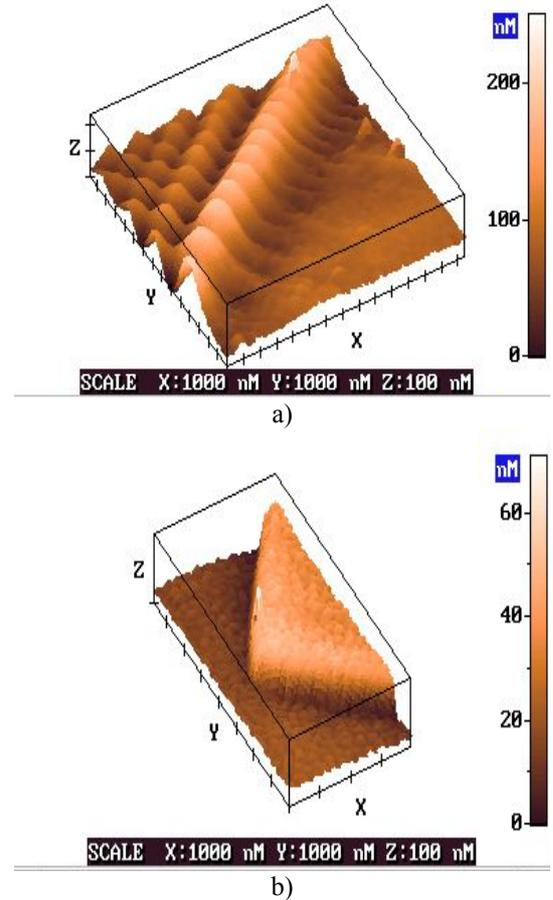
**Fig. 1.** a) 3D AFM picture of the pattern recorded on Se/ $As_2S_3$  nanolayered film with total thickness  $d=900\text{nm}$ , illuminated through a microgrid with 17mW, 532 nm diode laser for 30 min. b) 3D AFM picture of the pattern recorded on the same NLF due to the irradiation through a microgrid with 180 keV  $D^+$  ions, fluence  $1.6 \cdot 10^{16} \text{ ion/cm}^2$ .
