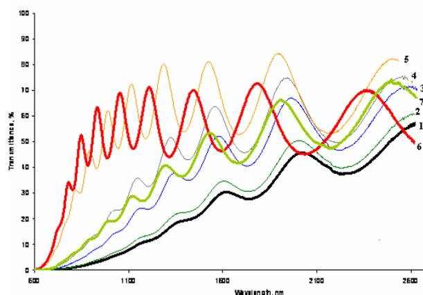
**Fig. 3.** Spectral dependences of the transmittance for as-deposited Bi/As<sub>2</sub>S<sub>3</sub> NML sample after 10 min annealing at 60 C (1), 80 C (2), 100 C (3), 120 C (4), 140 C (5) and 160 C (6) and for the same sample after laser irradiation with  $\lambda=635$  nm,  $P=30$  W/cm<sup>2</sup> (7).
